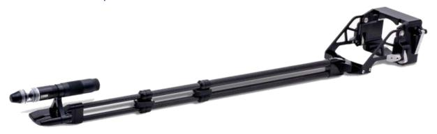
Our iPEK Laser ShapeScanner projects a ring of laser light onto the internal wall of the pipe, as the camera traverses down the pipe, providing a 3D cross sectional profile. The raw data can be viewed in real-time while on site, but is also recorded for further assessment.
